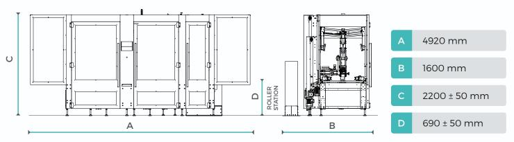
(Taping machine size for boxes W 600 H 600)
